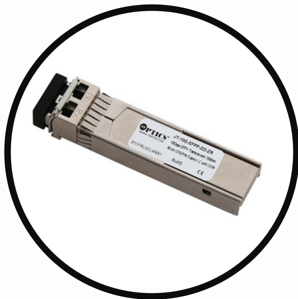
10G SFPP Transceiver 10GBASE-ZR 1550nm, 80km, DOM, LC, SMF JT-10G-SFPP-LC-ZR
