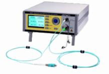
**Polarity Testing** Measure the polarity to ensure data from Tx at one end can be properly transmitted to Rx at
